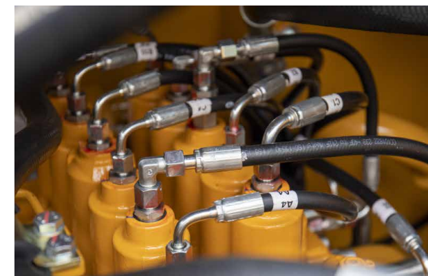
Main pump model: K7V125D Displacement: 2X130 CC Maximum flow: 2X273 L/min Rated pressure: 34.3 MPa
